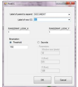
This operator will expand any parent EOC by adding childs EOC to it. These childs EOC will be connected component identified in the parent's XY bounding box. 2 binarization pre-treatment algorithms are possible. RANGEMAP\_XXX parameters will be useful for complex layouts with many blocks in the document; in this tutorial, default values are used.
